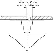
Clip the protective housing into position after the antenna has been mounted with the help of the three supplied screws.
