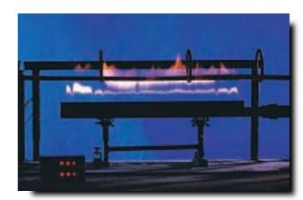
The samples are connected (via a 3 A fuse for each conductor) to a voltage source and tested at their rated voltage. All screens and other metal jackets are connected together and earthed. The conductors at the far end from the voltage source are bent apart in order to prevent them making electrical contact.
