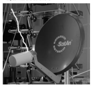
A former Kathrein LNB subjected to a lightning current test with 100 kA at the Bundeswehr University in Neubiberg near Munich.
