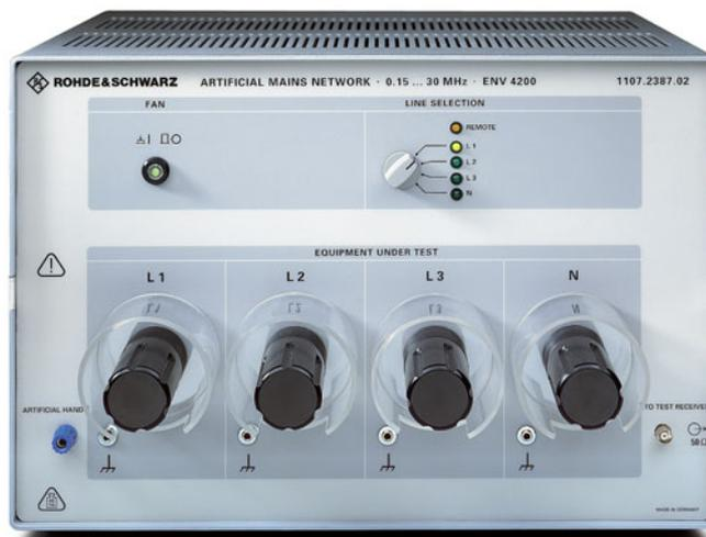
The maximum attainable current of the V-network is limited by the voltage drop at the standardized inductances (CISPR 16-1 prescribes the voltage drop at 5% of the AC supply voltage) and by unavoidable heat losses.
