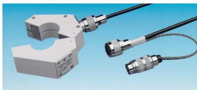
Model .02 with its extremely flat frequency response is optimal for current measurements as well as for measuring shielding effectiveness. Due to its high load capacity, model .03 is recommended for EMS measurements (bulk current injection). Thanks to their high magnetic overload capacity, these two models can be employed on power lines with currents up to 300 A without having an adverse effect on the measurement results.
