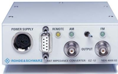
R&S® EZ-12 is a broadband matching unit for test receivers and spectrum analyzers with low-impedance inputs. It is used for high-impedance measurements of interference voltage at the feedpoint of a vehicle-mounted antenna in the long-, medium- and shortwave bands to VDE0879 Part 2 and CISPR25.
