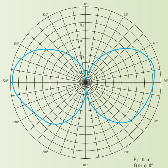
Typical elevation pattern at 120 MHz
