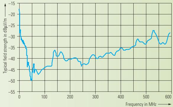
Typical field-strength sensitivity at antenna output (measurement bandwidth  $\Delta f = 1$  Hz;  $S/N = 0$  dB)
