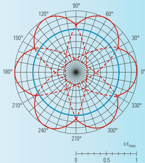
Typical horizontal omnidirectional reception characteristic (red = single patterns, blue = 3 dB reference) of a system with six R&S<sup>®</sup>HL410A3
