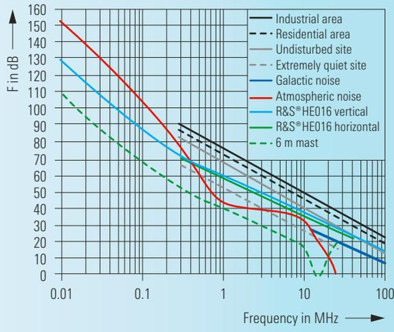
Typical inherent noise compared with different standard noise environments
