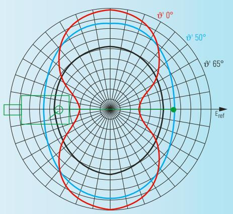
Azimuth patterns for various elevation angles  $\vartheta'$  with high-angle radiation
