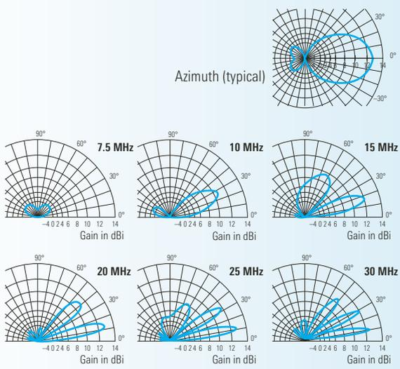
Typical radiation patterns on a 15 m mast
