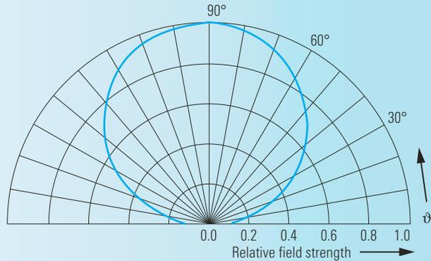
Coated wires, mast 10 m, ideal conductive ground
