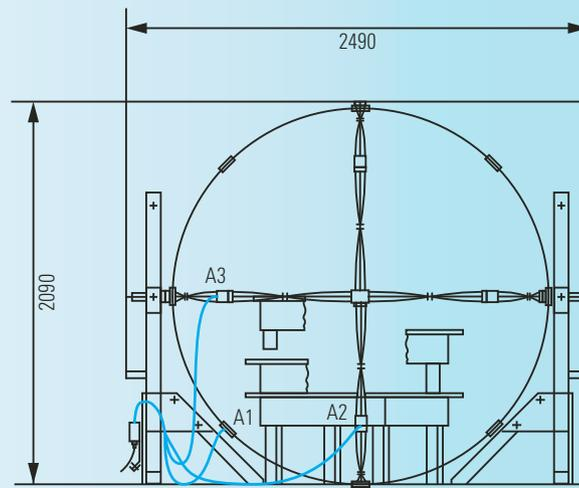
Dimensions adjusted to lower measurement height
