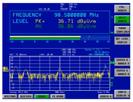
MIXED mode bargraph measurement and spectrum. The standard-conforming bargraph measurement and the fast sweep are displayed simultaneously
