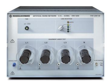
The maximum attainable current of the Vnetwork is limited by the voltage drop at the standardized inductances (CISPR 16-1 prescribes the voltage drop at 5% of the AC supply voltage) and by unavoidable heat losses.
