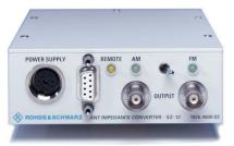
R&S<sup>®</sup>EZ-12 is a broadband matching unit for test receivers and spectrum analyzers with low-impedance inputs. It is used for high-impedance measurements of interference voltage at the feedpoint of a vehicle-mounted antenna in the long-, medium- and shortwave bands to VDE 0879 Part 2 and CISPR 25.
