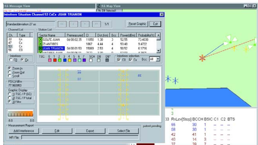
R&S®PCSD-K6 Evaluation Display (here TCH (Cx) with interference from another TCH (Cx))
