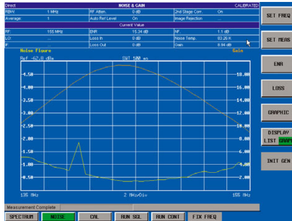
Measurements on a GaAs preamplifier show an anomaly at 140 MHz, whose cause is easily traceable in the spectrum analyzer mode
