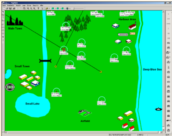
Fig. 8: Example of display of emitters on R&S® MapView during search operation with R&S® ScanLoc. Different types of emitters are shown with differently colored symbols. Known emitters (match with emitter data) appear with their names (here: Tac 1FR in the center). VHF/UHF DF stations are indicated by yellow circles
