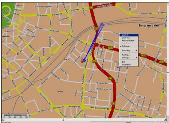
Display in a tracking DF system. Operation has been optimized for use without keyboard. The map is displayed in full-screen mode; by pressing a key, the displayed menu is shown with its main functions. The length of the DF beam depends of the level – short DF beam for high receive level
