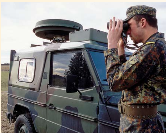
Vehicle setup – R&S®ADD195 DF antenna fixed to rooftop
