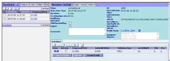
Fig. 22: Display of the classification result of a radio signal at 23 MHz (session detail). It automatically contains a link to possible objects that use the detected radio transmission method on this RF frequency for communications
