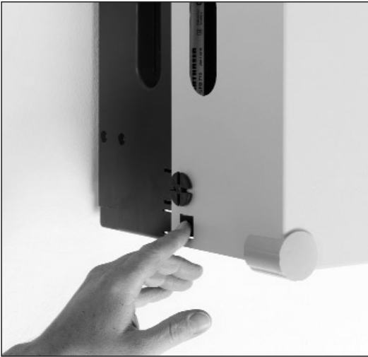
Unlock the cover of the UFO®DIGIplus unit by pressing the black locking button on the left side of the unit.
