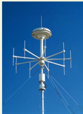
VHF/UHF DF antenna system (R&S®ADD153 (top), R&S®ADD050 (center), R&S®ADD070 (bottom))
