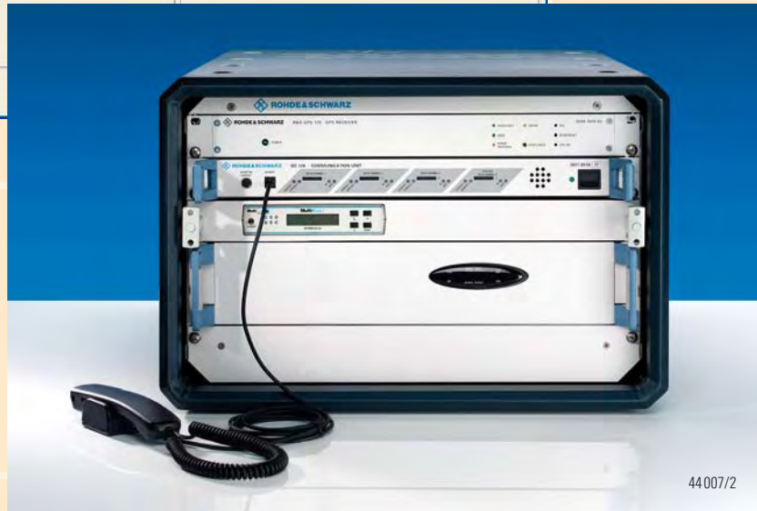
FIG 4 The monitoring system can be completely remote-controlled by using the Transportable Communication System R&S®TMS-C.
