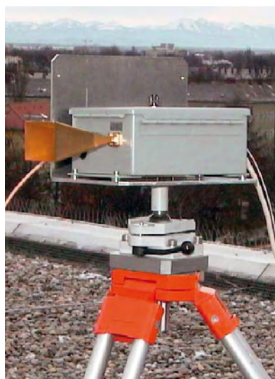
FIG 2 Five optional microwave converters expand the monitoring system for frequencies up to 110 GHz. You can easily mount a converter on a tripod, which is then ready to use.
