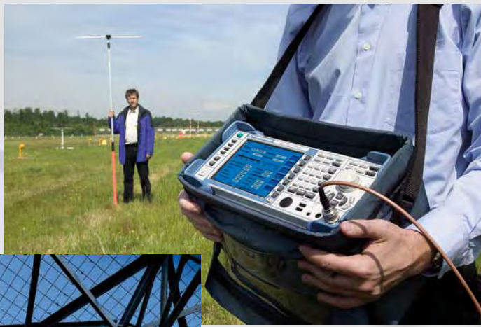
FIG 4 Static measurements in the field with the R&S®EVS 300 and the R&S®EVS-Z3 dipole antenna.
