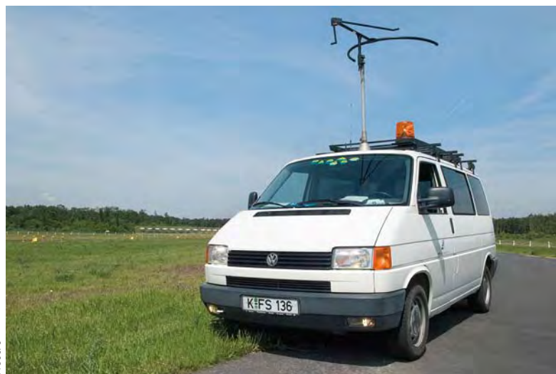
FIG 2 The measurement of ILS signals along the runways is performed by means of test vehicles, with the R&S®EVS300 as the core component.
