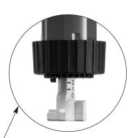
To set the downtilt angle exactly, you must look horizontally at the scale. The lower edge of the gearwheel must be used for alignment.
