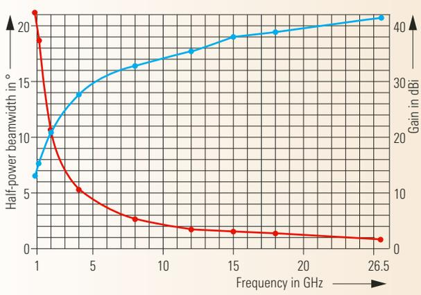
Typical gain (blue) and half-power beamwidth (red) of R&S® AC008 with feed R&S® HL050
