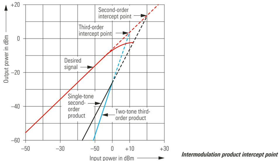
2. A point that is an extrapolated convergence – not directly measurable – of intermodulation distortion products in the desired output. That point indicates how well a receiver performs in the presence of strong nearby signals.
